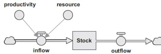
**Figure 1.** Example of a simple system dynamics stock-and-flow model
